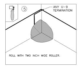
PS-15-E SURE-SEAL<sup>®</sup>/SURE-WHITE<sup>®</sup> PRESSURE-SENSITIVE INSIDE CORNER WITH CURED MEMBRANE
