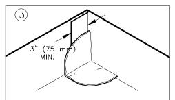
PLACE QUARTER SECTION ONTO DECK WITH LONG FOLDED SIDE FACING THE WALL. REMOVE REMAINING RELEASE PAPER. PRESS FIRMLY AND PROCEED WITH SECOND QUARTER GOING UP THE VERTICAL WALL BY PRESSING FIRMLY INTO CORNER.
