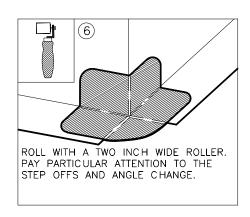
PS-15-F SURE-SEAL SURE-WHITE PRESSURE-SENSITIVE OUTSIDE CORNER WITH CURED MEMBRANE
