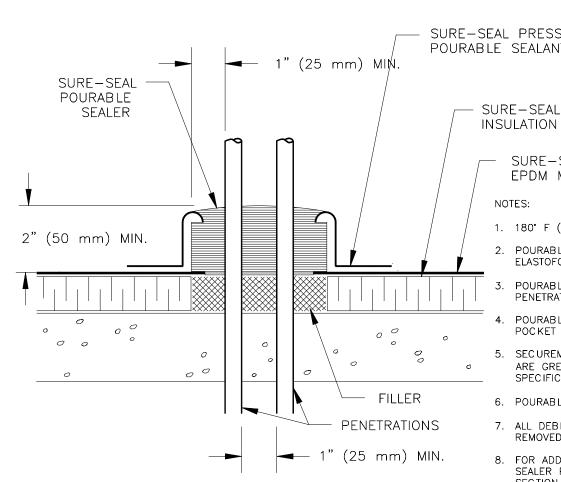
PENETRATIONS, MEMBRANE, FLASHING AND METAL DAM (INSIDE POCKET) MUST BE PRIMED PRIOR TO APPI YING POURABLE SEALER.
