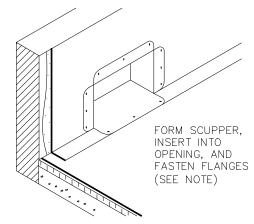
NOTE: FORM SCUPPER BOX OF PVC COATED METAL, TAPE THE METAL SEAM, AND OVERLAY WITH FLASHING BEFORE INSERTING INTO SCUPPER OPENING. POSITION THE SCUPPER BOX SO THE METAL SEAM IS LOCATED ON THE TOP OR SIDES OF THE SCUPPER.
