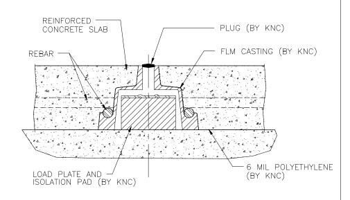
SLAB POSITION DURING CONCRETE CURE PERIOD N.T.S
