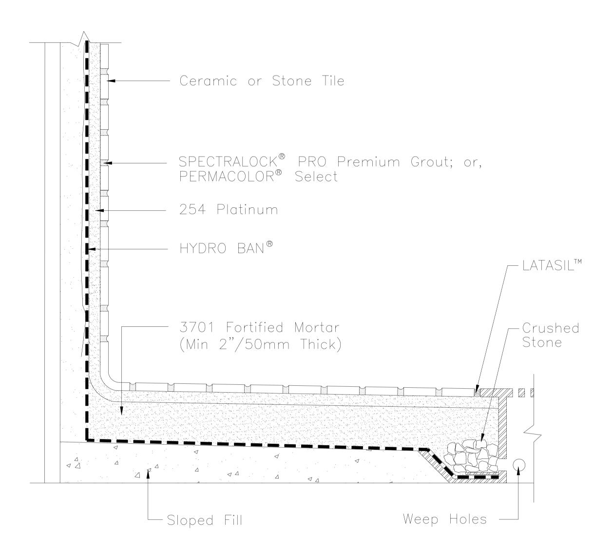
NOTE: Turn Up Waterproofing Membrane at Least 3" (76mm) Above Curb or Flood Point.
