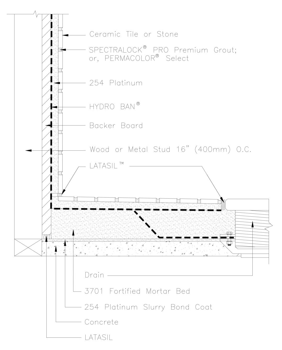
NOTE: HYDRO BAN to be installed to full height of tile on walls per TCNA.
