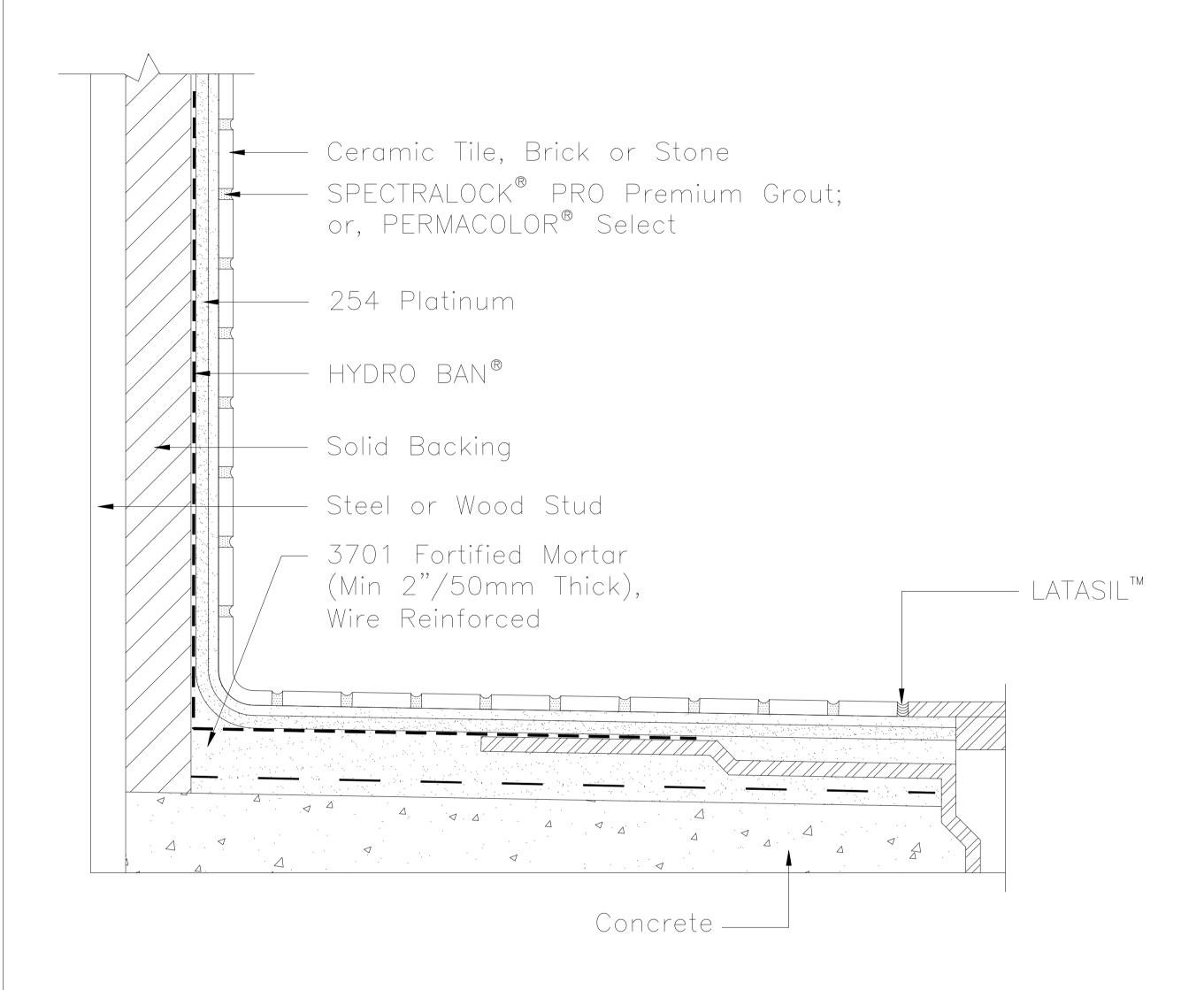
NOTE: HYDRO BAN to be installed to full height of tile on walls per TCNA.
