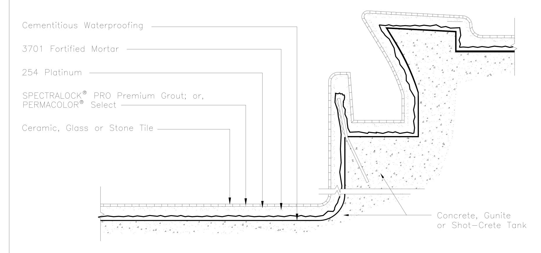
NOTE: Slurry Bond Coat of 254 Platinum is required under the mortar bed at all horizontal surfaces.
