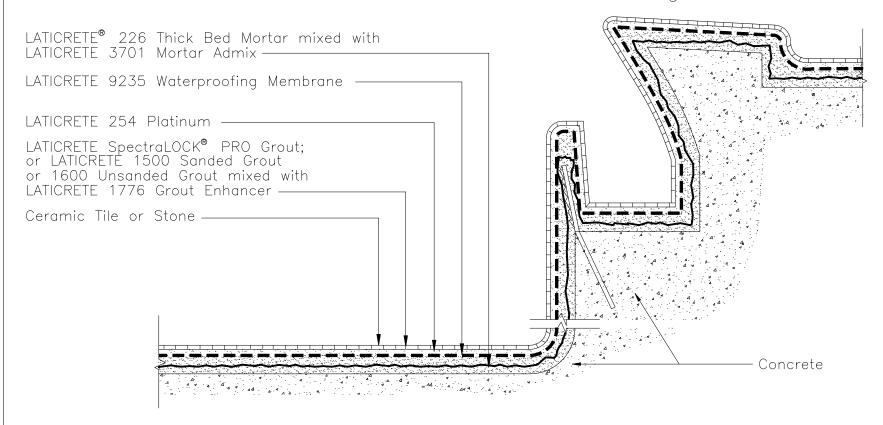
Note: Slurry Bond Coat of LATICRETE 254 Platinum is required under the mortar bed at all horizontal surfaces.
