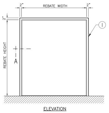
FRAME MUST BE INSTALLED AT FINISHED FLOOR HEIGHT.
