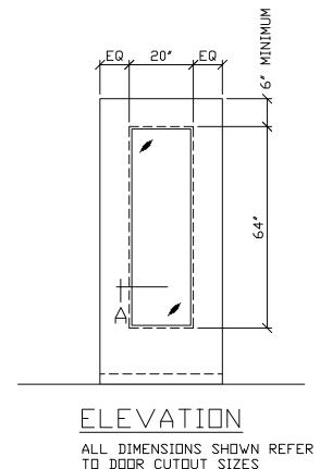
3/4" ACOUSTIC GLASS -1/4" CLEAR OR 1/4" GEORGIAN WIRE GLASS (PLEASE SPECIFY). WIRED GLASS WILL BE USED AUTOMATICALLY IF THE OPENING 1/4" CLEAR GLASS -IS FIRE RATED FIXED STOP ON THE SECURE-REMOVABLE STOP SIDE (LOCK CYLINDER SIDE) OF THE DOOR
