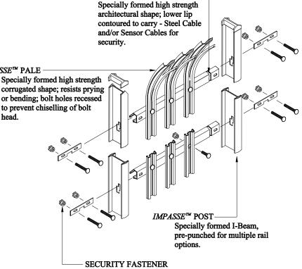
Stainless steel security nut prevents tampering or removal by normal tools.
