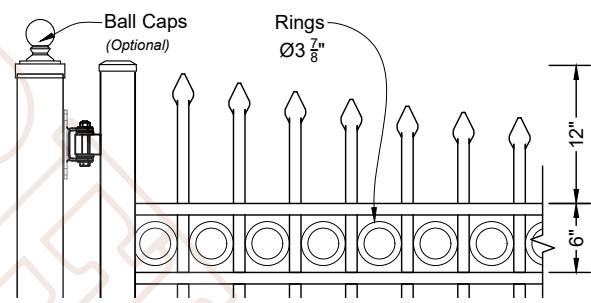
**A** 04 Rings Welded To Pickets Scale: NTS
