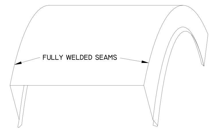
ALUM. "ARCHED" SNAP-TIGHT COPING W/ 8" CONCEALED JOINT COVER PLATES WELDED TO THE "UPPER END" OF THE ARCHED PIECE
