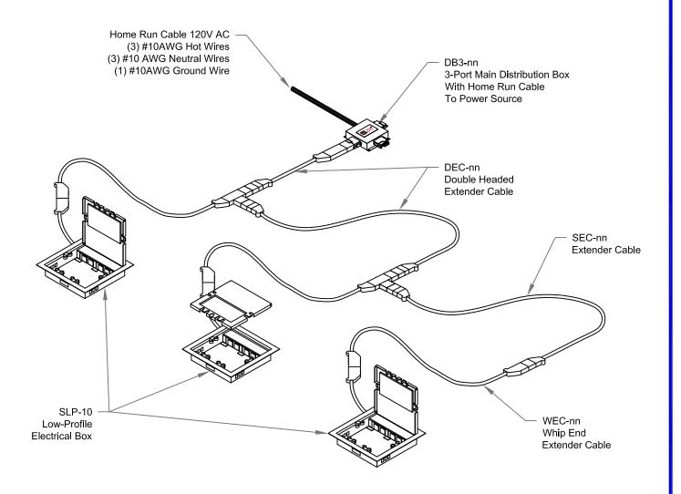
The DB3-nn 3-Port Main Distribution Box Has Three (3) 20A/120V Circuits Available. The Above Illustration Shows A "Daisy Chain" Application On One 20A Circuit Only
