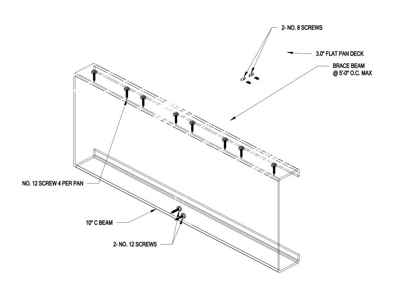
3.0" FLAT PAN DECK TO 10" C BEAM AND BRACE
