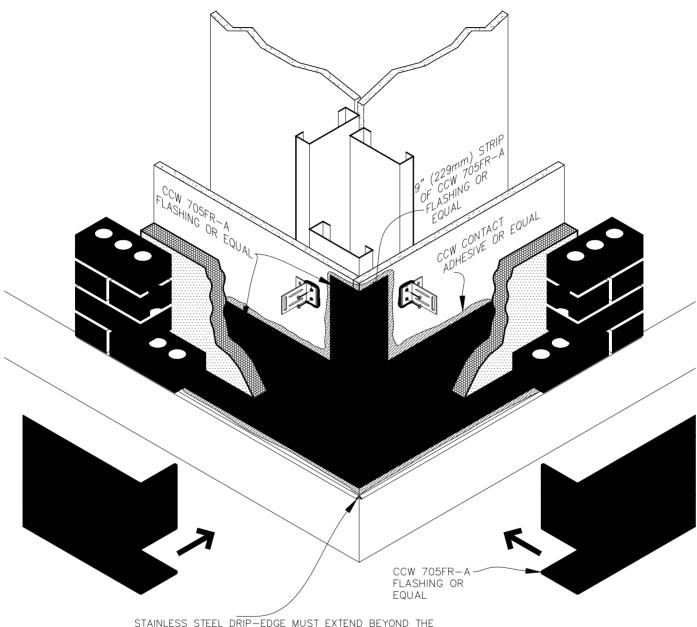
STAINLESS STEEL DRIP-EDGE MUST EXTEND BEYOND THE FACE OF EXTERIOR CLADDING. SET IN HEAVY BEAD OF SEALANT OR CONTINUOUS STRIP OF 1" (25mm) WIDE BUTYL TAPE.
