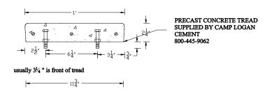
3/8" BOLTS ENCASED IN CONCRETE W/ SUPPORT NUT
