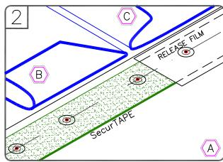
FOLD SHEETS BACK AS SHOWN. APPLY EPDM PRIMER TO THE SPLICE AREA ON BOTH SURFACES AND ALLOW TO FLASH-OFF. APPLY SecurTAPE WITH RELEASE FILM ALIGNED WITH PRE-MARKED LINE.
