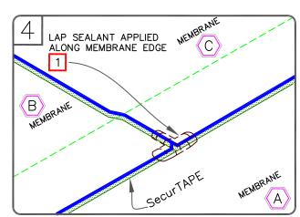
SPLICE SHEET C TO SHEET A AND B, PRESS TOP SHEET ONTO BOTTOM SHEET USING HAND PRESSURE TOWARDS THE OUTER EDGE OF THE SPLICE AND ROLL THE SPLICE AREA WITH A 2" (5cm) WIDE STEEL ROLLER.
