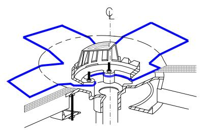
EXTEND THERMOPLASTIC MEMBRANE ONTO MEMBRANE SECTION POSITIONED AT DRAIN SUMP AND CUT AS SHOWN TO LAY FLAT IN SUMP. HOT AIR WELD A MINIMUM OF 1-1/2" (4cm) COMPLETELY SURROUNDING AREA.
