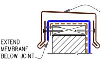
METAL CAP (BY OTHERS), SLOPE DOWNWARD TOWARDS ROOF
