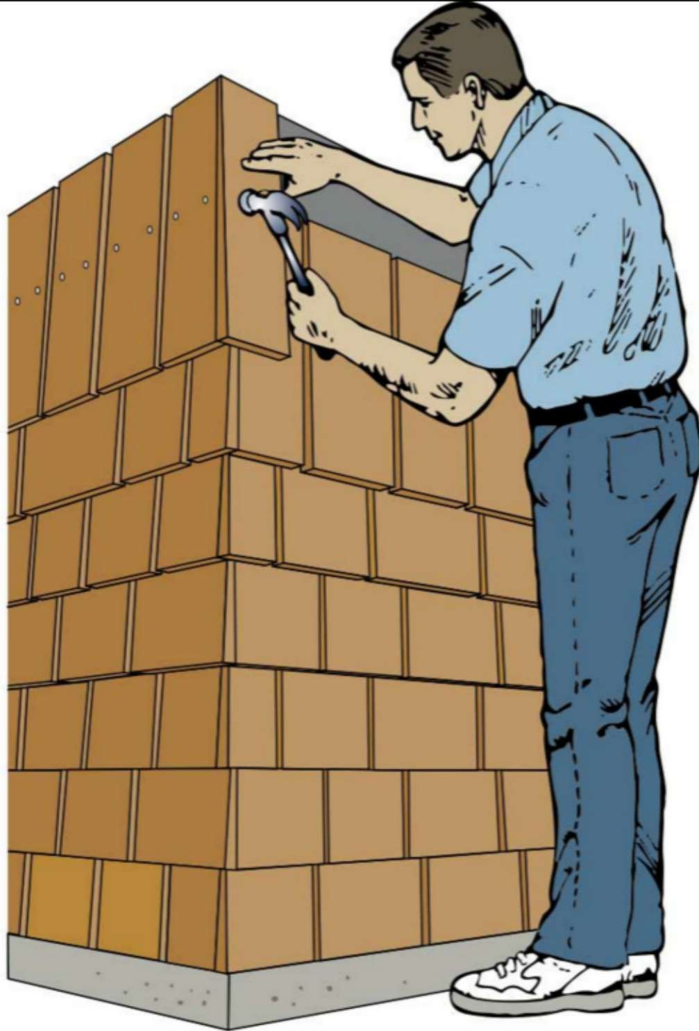
Figure 9: Fitting Laced Corner Courses
