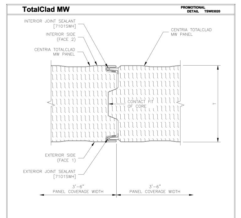
NOTES: 1. IF JOINT SEALANTS ARE REQUIRED, THEY ARE SPECIFIED AS A SILICONE SEALANT IN ORDER TO CONFORM TO THE PANEL'S ASTM E-119 FIRE RESISTANCE RATING. SEALANT IS REQUIRED IN BOTH JOINTS IF THE PANEL IS EXTERIOR AND EXPOSED TO WIND AND DRIVEN RAIN.
