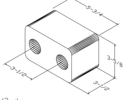
TB-20 is molded from a nylon & polyester fibre reinforced rubber of 80 (+ or -) 5 durometer, and has an average impact resistance of 95% under ASTM 1170.
