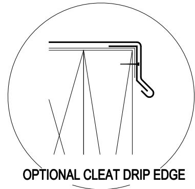
ONE METAL PAN FLASHING WITH DRIP EDGE
