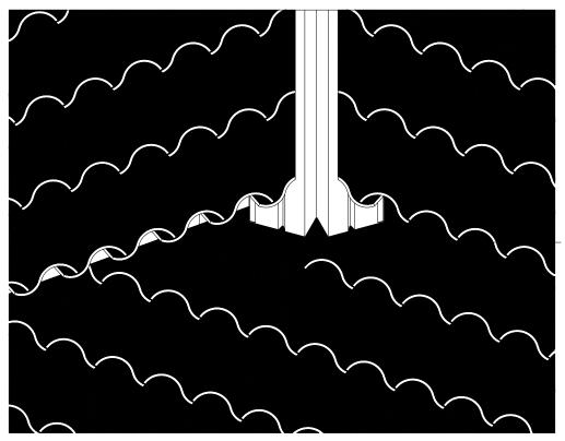
THE VALLEY MUST LAP ONTO THE TILE OF THE COURSE BELOW THE ROOF TRANSITION
