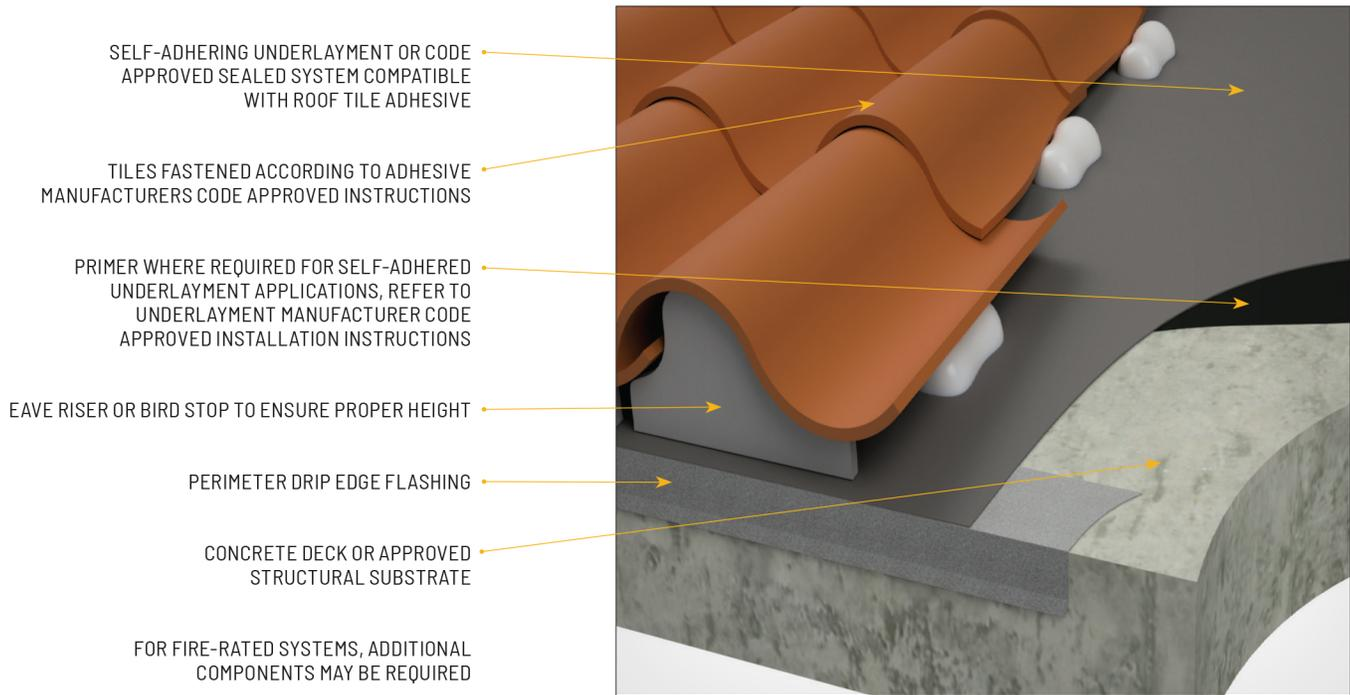
NOTE: ADHESION OF UNDERLAYMENT TO SUBSTRATE SHALL BE IN ACCORDANCE WITH ASSEMBLIES RECOGNIZED IN A CURRENT ICC-ES EVALUATION REPORT FOR ROOF TILE ADHESIVES EVALUATED TO THE REQUIREMENTS OF AC-152.
