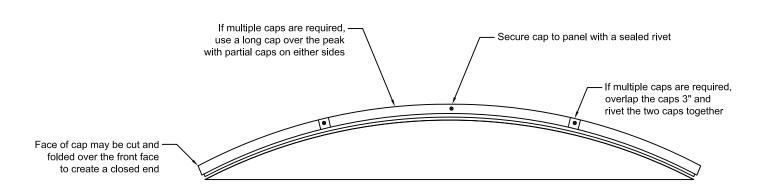
Note: Details such as ridge, eave, clips, etc. have been omitted from this drawings for clarity. See full set of standard details for those areas.
