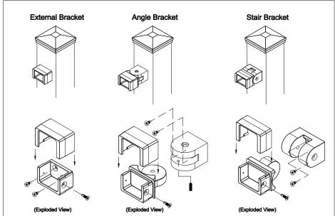
NOTE: Bracket to Post Connection: T25 3/4" Thread Cutting Screw Ralling Panel to Bracket Connection: T25 3/4" Thread Cutting Screw
