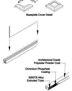
NOTE: Bracket to Post Connection: T25 3/4" Thread Cutting Screw Railing Panel to Bracket Connection: T25 3/4" Thread Cutting Screw
