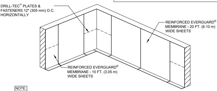
1. FIRST SHEET FROM THE CORNER AND FIRST SHEET FROM THE WALL EDGE REQUIRE A ROW OF DRILL-TEC $^{\text{IM}}$  PLATES AND FASTENERS 12" O.C. MID WAY UP THE WALL AS SHOWN. CORNER AND EDGE SHEETS ARE 10' (3.05 m) ALL SHEETS IN BETWEEN ARE 20' (6.10 m) WIDE.
