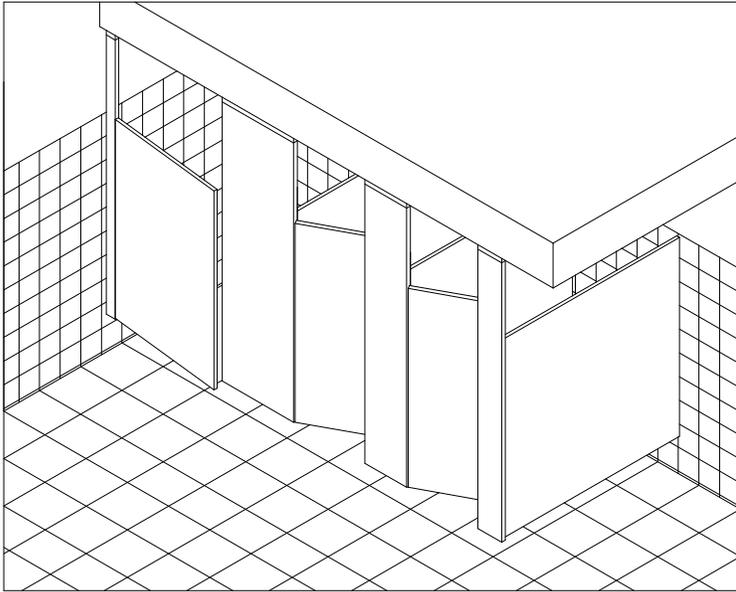
Scope - Stainless Steel toilet partitions are constructed of two sheets of satin stainless steel bonded together before attaching die drawn molding on all four sides of panels. Mitered reinforcements fused to corners for added structural strength. Fillers shall be General's Ribcore sound-deadening insulation.
