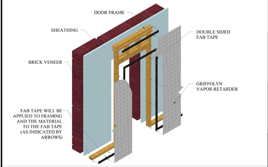
NOTE: This document provides information related to the installation of "Fab Tape", Vapor Retarder and related components. The information provided is recommended options for securing Griffolyn Vapor Retarder on an interior wall. The orientation or location of Griffolyn Vapor Retarders in a wall construction is as specified by the architect or specifier.
