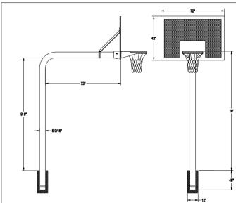
Pole shall be constructed of 5 8/16" outside diameter schedule 40 structural pipe and have a hot dipped galvantzed finish. Design shall be a best gooseneck style and allow for a 45" bury into the ground and a 72" extension from the front of the pole to the tipe of the buckboard. The 56" diameter, 7 ag. five created galvantzed studies broses shall support the top of the backboard or the pole to the tipe of the t
