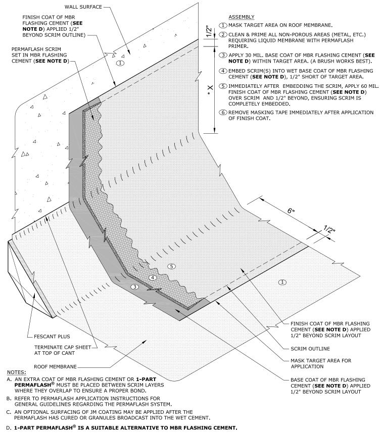
JM PERMAFLASH STANDARD CANTED BASE FLASHING DETAIL
