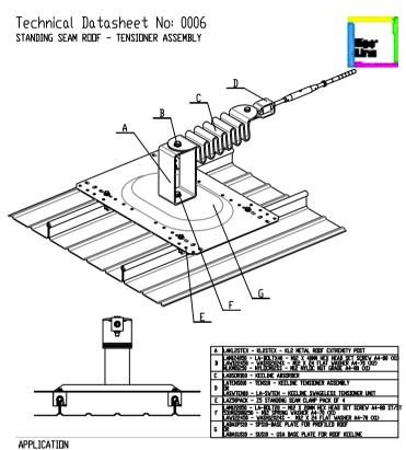
The Energy Absorber is designed to dissipate the energy generated throughout the system and reduce the end loadings to below 2248lbs. The pretension indicator is a way of instantly adjusting and checking the correct tension of the life line cable.
