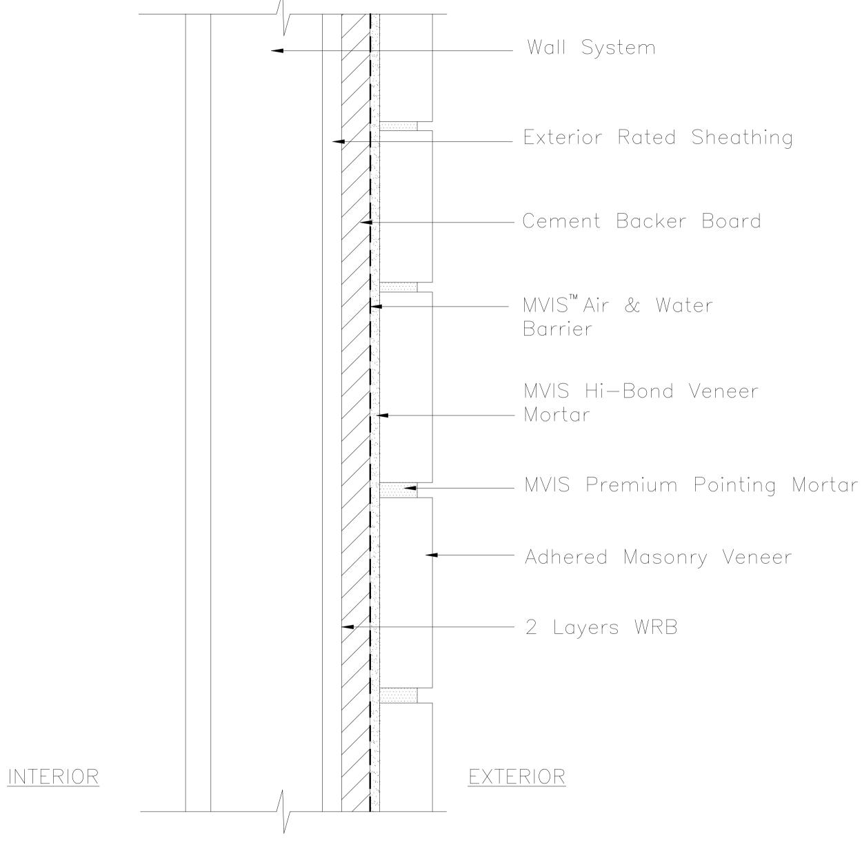
NOTE: Vapor Barrier, Air Barrier, Water-Resistive Barrier, Waterproofing Membrane, Flashing, Cleavage Membrane, and Insulation type and locations to be determined by design professional. See full MVIS specification for additional design considerations.
