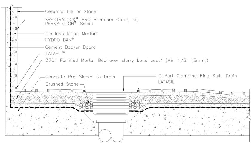
\* Slurry bond coat and tile installation mortar to be either 254 Platinum, 257 TITANIUM™ or MULTIMAX™ LITE.
