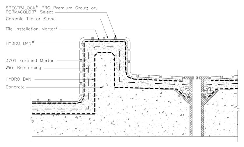
\* Tile installation mortar to be either 254 Platinum, 257 TITANIUM<sup>™</sup> or MULTIMAX<sup>™</sup> LITE. Pre-formed curbs are acceptable.
