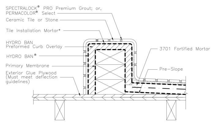
\* Tile installation mortar to be 254 Platinum, 257 TITANIUM™ or MULTIMAX™ LITE.
