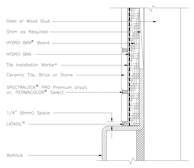
\* Tile installation mortar to be either 254 Platinum, 257 TITANIUM™ or MULTIMAX™ LITE.
