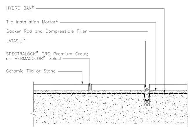
\* Tile installation mortar to be either 254 Platinum, 257 TITANIUM or  $\mathsf{MULTIMAX}^\mathsf{T}$  LITE.
