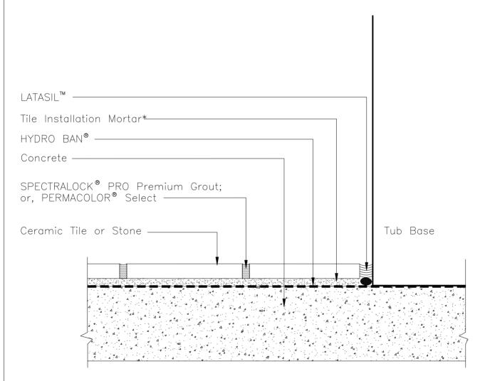
\* Tile installation mortar to be either 254 Platinum, 257 TITANIUM or MULTIMAX LITE.
