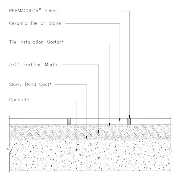
\* Slurry bond coat and tile installation mortar to be either 254 Platinum, 257 TITANIUM™ or MULTIMAX™ LITE.
