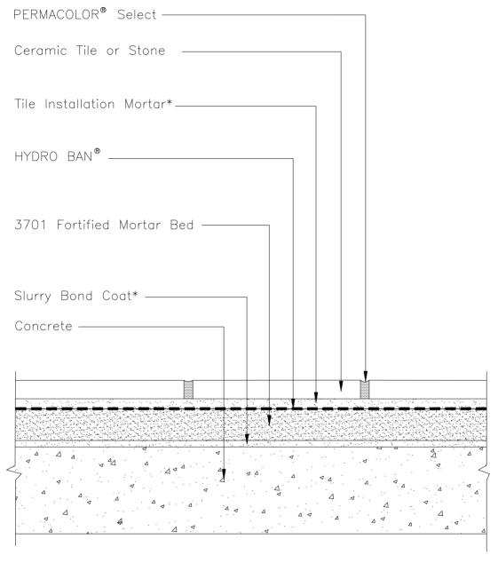
\* Slurry bond coat and tile installation mortar to be either 254 Platinum, 257 TITANIUM™ or MULTIMAX™ LITE.
