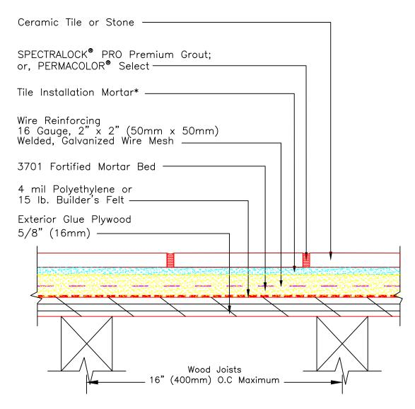
\* Tile installation mortar to be either 254 Platinum, 257 TITANIUM<sup>™</sup> or MULTIMAX<sup>™</sup> LITE.
