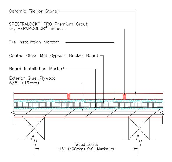
\*Board Installation Mortar and Tile Installation Mortar to be either 257 TITANIUM, 254 Platinum, or MULTIMAX LITE.
