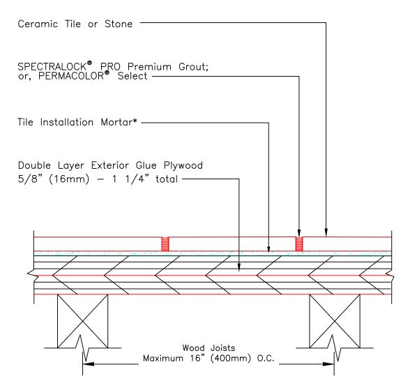
\* Tile installation mortar to be either 254 Platinum, 257 TITANIUM™ or MULTIMAX™ LITE.
